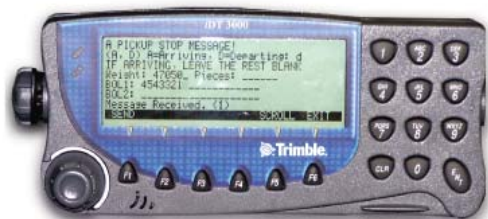
The Trimble iDT is the in-vehicle display device used with the Trimble GeoManager FlexForms Interface for TMW
